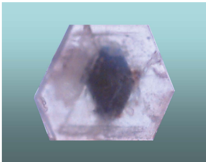
Figure 1 Image of the crystal obtained by seeding the saturated solution of (2) with crystals of (1). The inner part contains the blue–violet \text{Co}^{\text{II}} complex; the outer part is composed of the colourless \text{Zn}^{\text{II}} complex.
